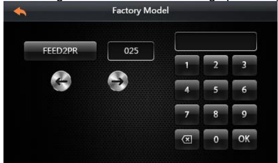
Fig.46 14·Setting the max value for feeding speed 3 (Fig. 47)
