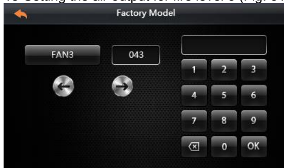
Fig.51 19 Setting the air output for fire level 4 (Fig.52)
