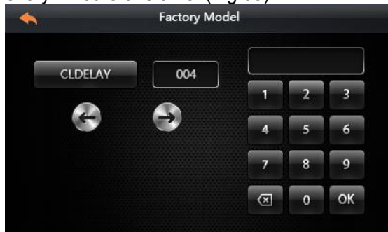
Fig.53 21·Setting the time delay of feeding after successful ignition, for example: start to feeding the pellet in 120s
