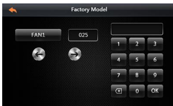
Fig.49 17·Setting the air output for fire level 2 (Fig. 50)
